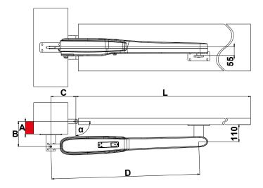
Compatible with CAME ATI 5000 brackets (with standard ATI/AXI/AXO CAME adapter) Compatible with column bracket of NICE TOONA 5 (use KING EVO L leaf bracket)
