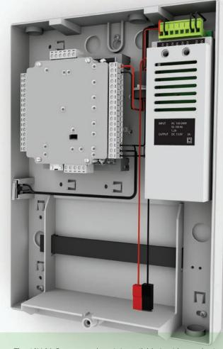
The 12V 2A Power supply unit is available in either a plastic or metal cabinet. The cabinet can house both the 12V 2A PSU and a Net2 or I/O ACU with the option to accomodate a 12V/7Ah back up battery if desired. A tamper switch is also installed which registers an alarm if the lid is opened when connected to an ACU or I/O board. Please note that the Net2 nano ACU and I/O board are not available for integration within the metal cabinet.
