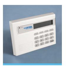
The LNL-CK Lenel Command Keypad integrates a 32-character backlit LCD display with a 16-position keypad and a reader port. The command keypad serves as a command reader, a reader from which user commands can be issued to execute local I/O functions. Reader command programming is accomplished using the OnGuard System Administration application.
